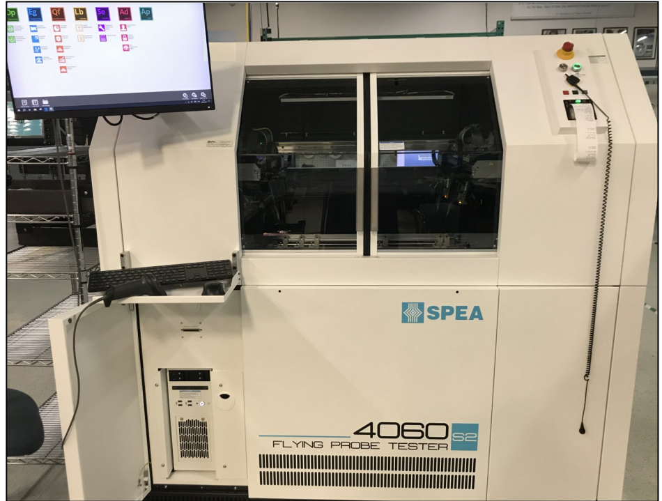
Above, the SPEA 4060 flying probe tester provides a comprehensive fixtureless test solution. Below, a PCBA under test.
