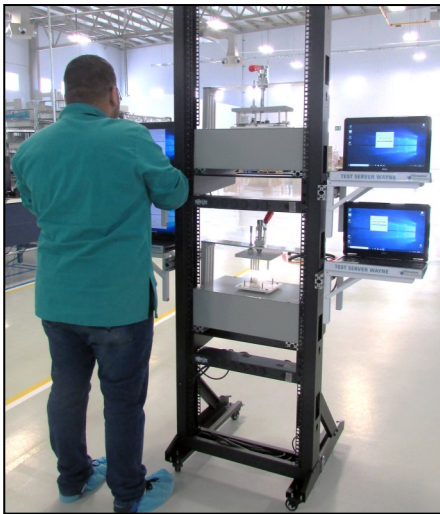
The redesign on this test unit quadrupled units under test and reduced the test station footprint from 72 sf to 6 sf.
