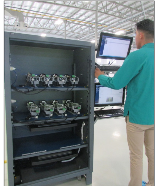
The redesigned burn-in cabinet can now test eight units simultaneously.
