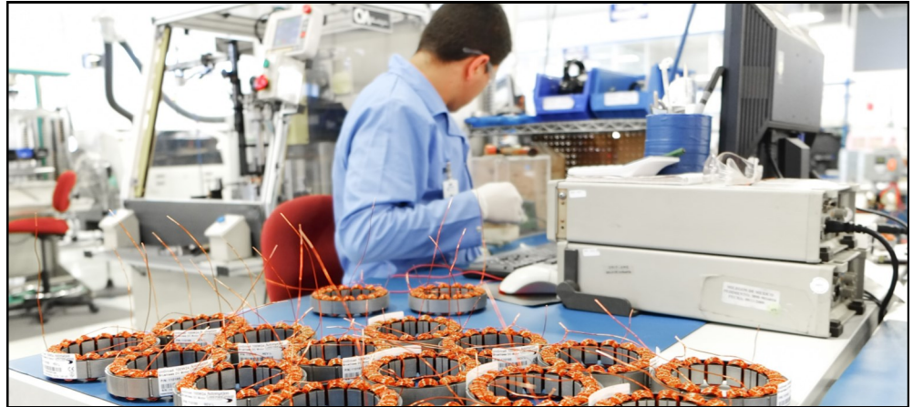
A specialized work cell for brushless DC (BLDC) motor production.
