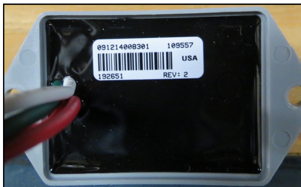
The unit is potted to protect the electronics.
